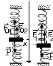
$$\text{Ta có: } F = F_1 + F_2, \text{ vậy: } \left[ k_{\text{hệ}} = k_1 + k_2 \right], \text{ chu kỳ: } T = 2\pi \sqrt{\frac{m}{k_{\text{hệ}}}}$$
