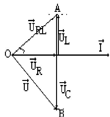
$$\text{Từ đó: } \varphi_1 + |\varphi_{u/i}| = \frac{\pi}{2}, \text{ vì } \varphi_1 < 0, \varphi_{u/i} > 0 \text{ nên: } \tan \varphi_1 = -\cot \varphi_{u/i} = -\frac{1}{\tan \varphi_{u/i}}$$
